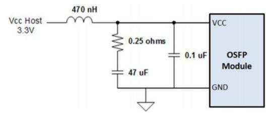
Figure 4. Recommended Power Supply Filter
