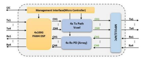
Figure 1. Transceiver Block Diagram
