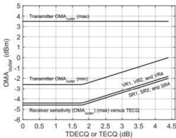
**Figure 6. Illustration of Receiver Sensitivity Mask for 400G-VR4**
